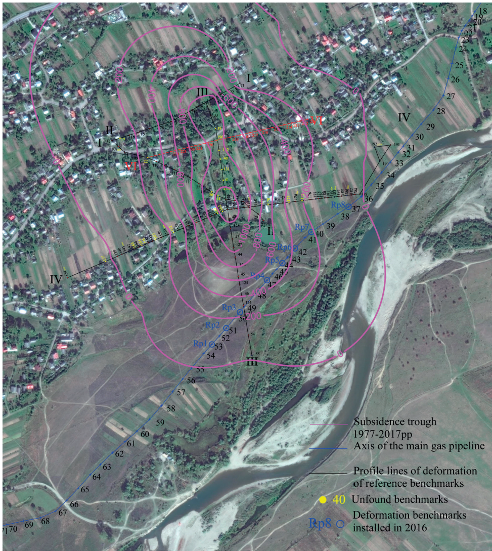
Figure 5. Map of the locations of ground benchmark profile lines, axis of the main gas pipeline and subsidence troughs
